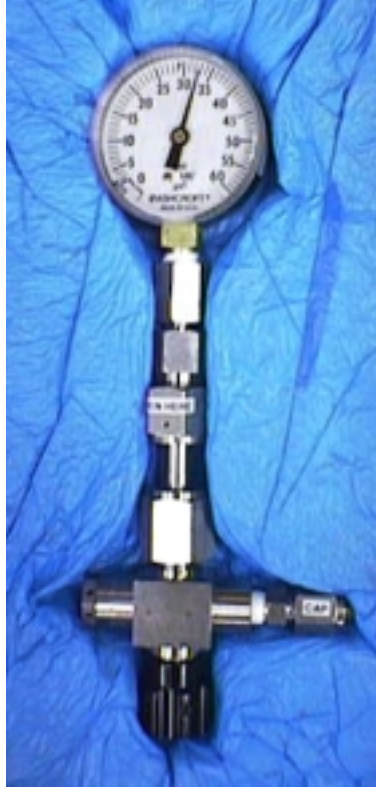
Fig. 1-3. This vessel can be safely used to ship and store a capsule under pressure until the capsule is removed just before shot time. The pressure vessel is more reliable and easier to use than the previous technique of keeping the capsule cooled by dry ice.
