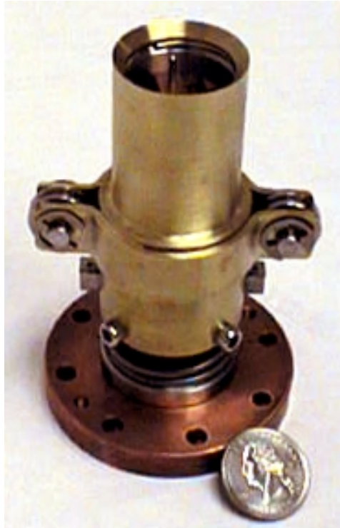
Fig. 5-23. The parts of the cryogenic target gripper have been machined. The gripper is shown partially assembled.
