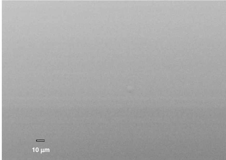
Fig. 2-12. SEM photomicrograph of the surface of a 12\ \mu\text{m} \times 2\ \text{mm} PAMS mandrel coated with 70\ \mu\text{m} of Ge-GDP. The shell surface is virtually dome free.
