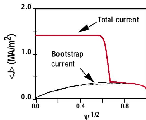
Fig. 5. Self-consistent current profile from high  $\beta$ , high  $I_i$  equilibrium  $\beta_N = 4$ ,  $I_i = 1.2$ ,  $q_{95} = 8$ ,  $q_0 = 1.05$ .
