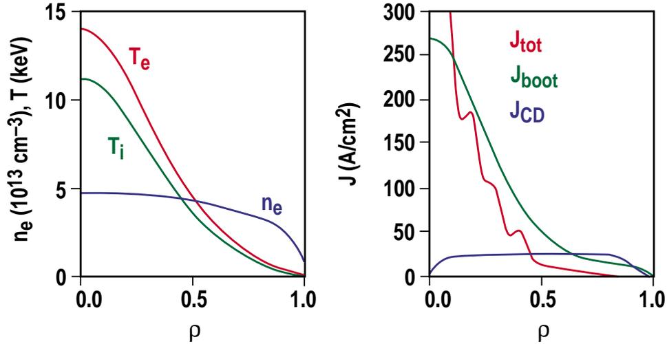
Fig. 12. A high  $I_i$  steady-state with  $\beta_N H > 10$  can be sustained by a 3 MW ECH system. The parameters are:  $B = 1.9$  T,  $I_i = 1.6$ ,  $\beta_N = 2.5$ ,  $I_{BS} = 0.41$  MA,  $I = 1.0$  MA,  $\beta_N = 4.0$ ,  $P_{FW} = 3.6$  MW,  $I_{FW3} = 0.17$  MA,  $q_0 = 0.55$ ,  $H = 3.0$ ,  $P_{EC} = 2.4$  MW,  $I_{EC} = 0.14$  MA,  $q_{95} = 5.6$ ,  $n = 4.2 \times 10^{13}$  m<sup>-3</sup>,  $P_{NB} = 5.0$  MW,  $I_{NB} = 0.27$  MA.
