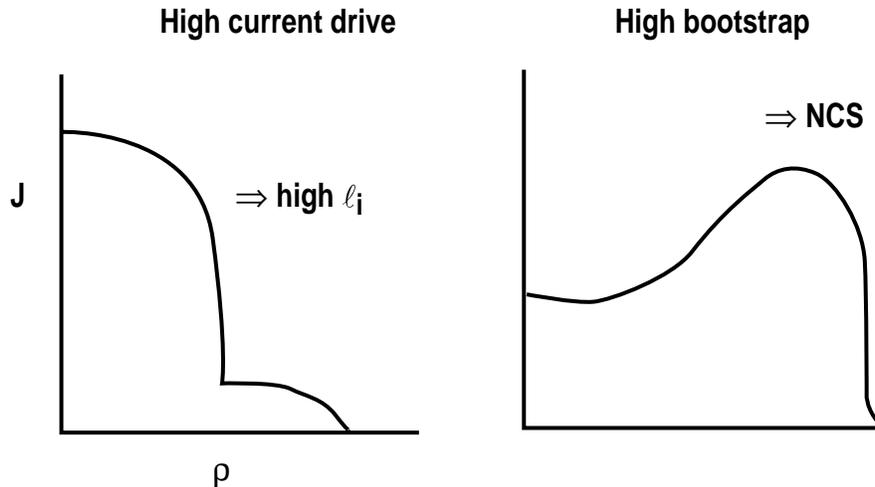
Fig. 1. Steady state considerations also lead to two “natural” current profiles.
