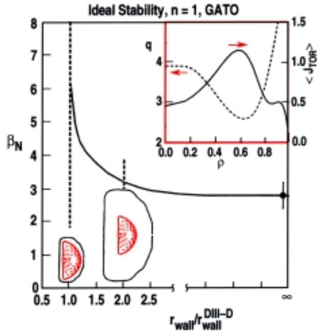
Fig. 3. Maximum stable beta increases for closer wall position: ideal  $n=1$  stability using DIII-D plasma shape and DIII-D wall. Insets are typical current density and  $q$  profile (Taylor1995).
