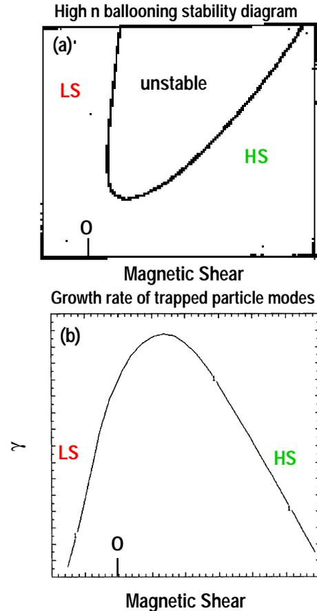
Fig. 2. Both low magnetic shear (LS) and high shear (HS) are favorable for: (a) higher beta, (b) reduced turbulence and reduced transport. Magnetic shear is  $s \propto R/B_T^2 q^2 dp/dr$ .
