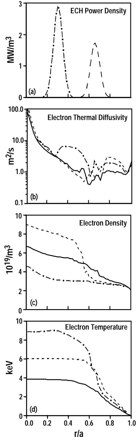
Fig. 9. ECH barrier control is illustrated by a three-case comparison: 6 MW NBI only (solid), 6 MW NBI + 6 MW ECH at  $r/a \sim 0.7$  (dashed), 6 MW NBI + 6 MW ECH at  $r/a \sim 0.3$  (dot dashed). Shown are profiles of (a) ECH power density, (b) model electron thermal diffusivity, (c) electron density, and (d) electron temperature.
