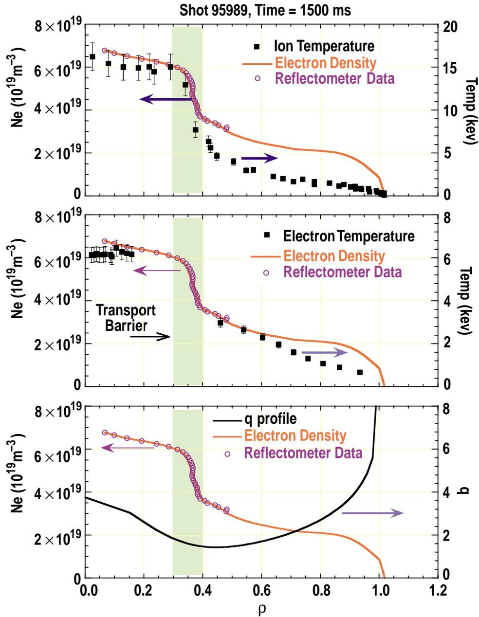
Fig. 10. Transport barrier in the density.
