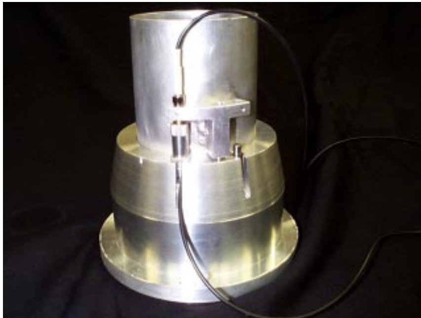
Fig. 5-10. Picture of the assembled parting optical fiber connection.
