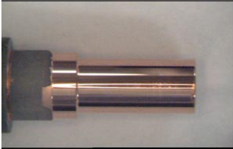
Fig. 1-2. A typical central can mandrel with a copper coating.
