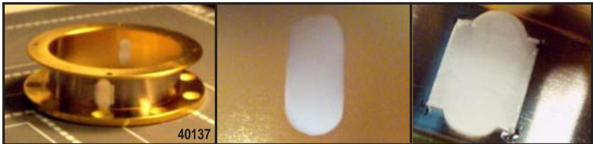
Fig. 3-5. A new application for low density foams is shown here. The photograph on the left is an overview of a current return can with two hole closure foams. The inner diameter of the can is approximately 51 mm. Close-up views of the foams are shown on the right side. The inside view confirms that there is no foam protruding into the can where it could interfere with other target components. The outside view documents the method of securing the foam. The 11 by 4 mm oval is cast with thin side extensions that can be tacked in place with four drops of epoxy — one at each corner. The epoxy is far from the hole so that it is not seen by any diagnostic.
