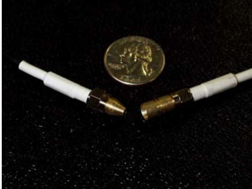
Fig. 5-9. Picture of the conical fittings attached to SMA connectors.
