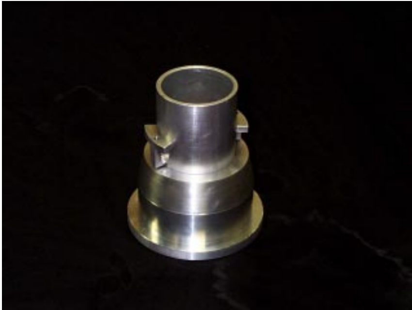
Fig. 5-8. Picture of the parting joint mockup.
