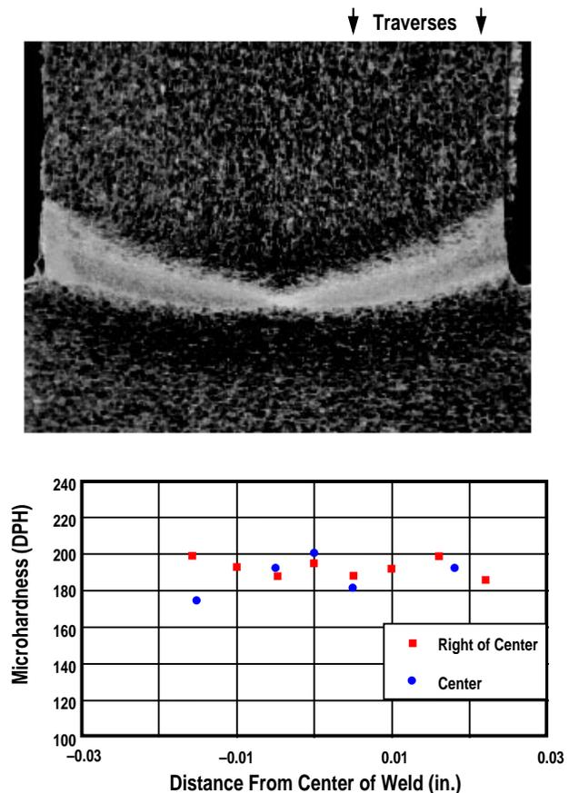
Fig. 4. Etched cross-section of V-5Cr-5Ti alloy inertia weld trial sample showing location of weld joint and microhardness measurements.
