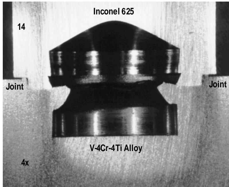
Fig. 5. Ground cross section of inertia-welded V-4Cr-4Ti alloy (bottom)/Inconel 625 (top) joint in simulated tube-tube configuration. Note: indentation and inward plastic flow of original V-alloy surface and inward flow (buckling) of tubular Inconel 625 lip.
