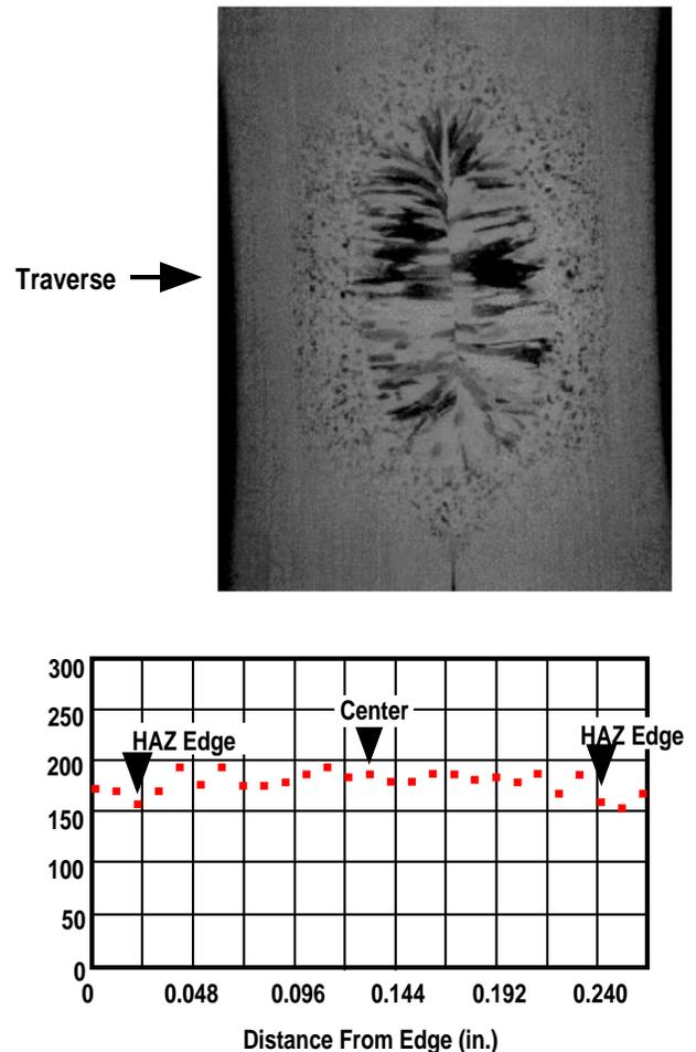
Fig. 3. Resistance spot weld of 3.8 mm thick V-Cr-4Ti alloy sheets with microhardness profile across the weld nugget.
