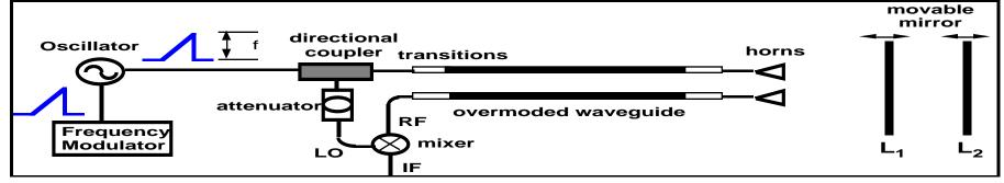
• Frequency sweep and path length difference between microwave paths leads to frequency difference
