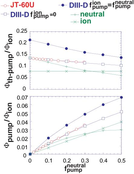
Data for JT-60U are plotted as a function of pumping ratio at the throat.
