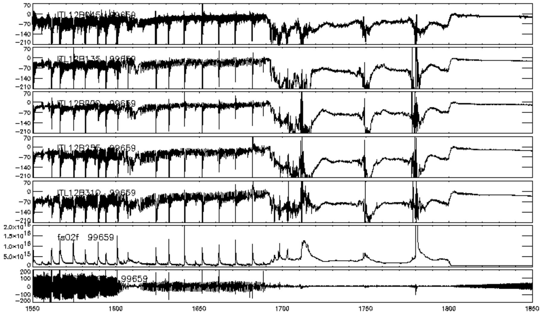
**Fig. 6** Current through five tiles in Ring#12B around a period of magnetic activity.  $D_\alpha$  and Mirnov signals are also shown at bottom.
