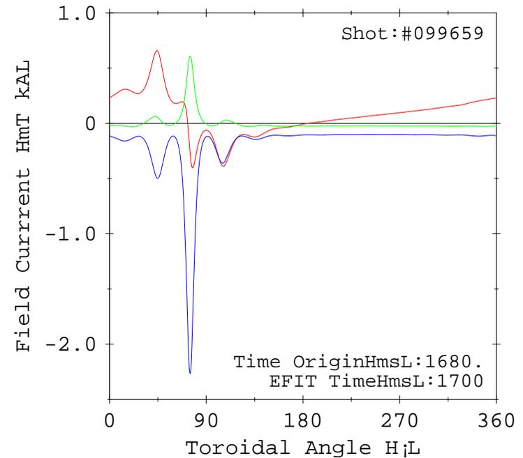
**Fig. 16** Toroidal variation of field is obtained by rotating either the line current or the sensors. Field shown here is for a unit current (1 kA).
