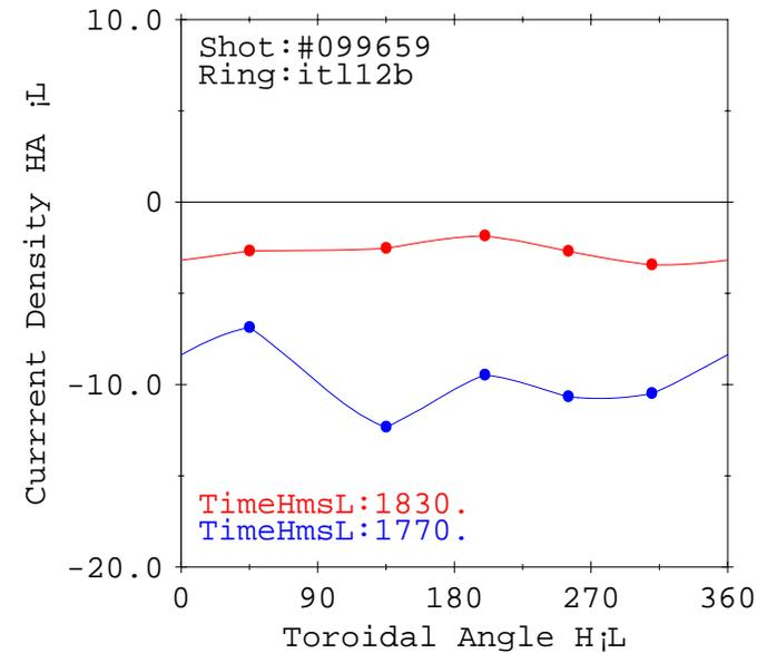
**Fig. 12** Current can be fairly axisymmetric in some parts of an RWM event. It is closely axisymmetric after an RWM.
