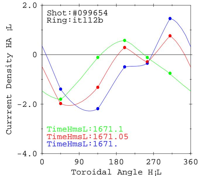
**Fig. 14** Two toroidal ‘nodal’ points are evident as if in a **standing wave** pattern, one around 45 deg (here at a finite amplitude!) and the other around 270 deg. Apparent progressive phase inbetween seems to suggest, however, a **travelling wave** pattern — a curious situation.
