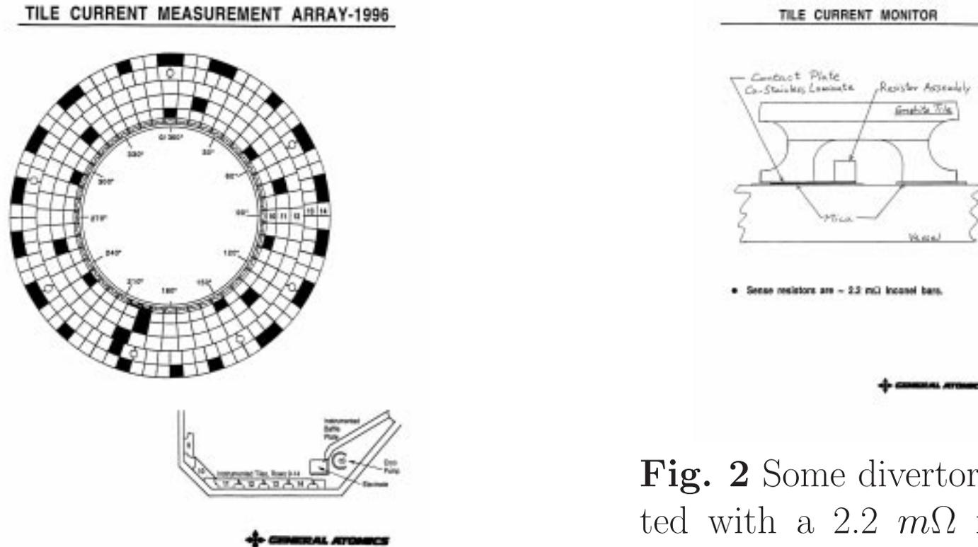
**Fig. 1** Divertor bottom tiles are laid in rings. Forty eight tiles in **Ring#12B** carries most current (for this study). Each tile spans 7.5 deg toroidally and 13.9 cm radially. The data system bandwidth is 15 kHz for the tile current diagnostic, and is significantly slower than for the Mirnov and  $D_\alpha$  systems referred to later.
