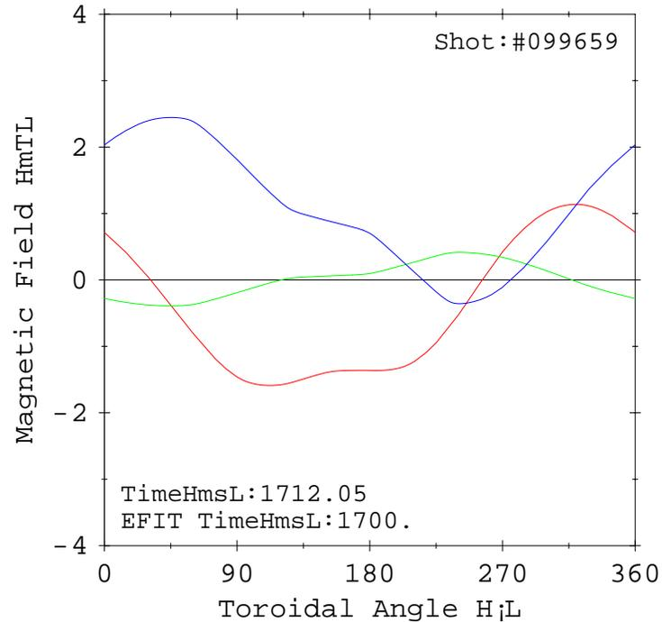
**Fig. 19** Toroidal variation, up to a few **tens of Gauss at spiky peaks** (here nearly 30 G) and **several Gauss between peaks**, is comparable to structural error fields associated with locking MHD modes, and is large enough to account for parts of field attributed to LM's and RWM's.
