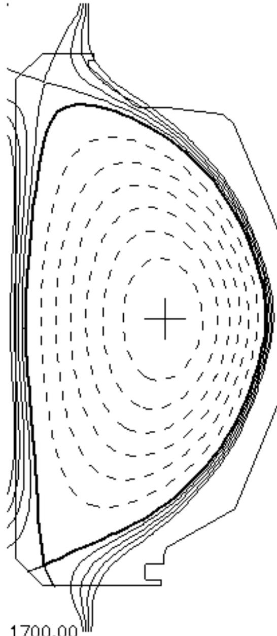
**Fig. 5** Parameters and flux surfaces of a typical equilibrium studied. Flux surfaces in SOL intersect tiles in Ring#12B and other rings.
