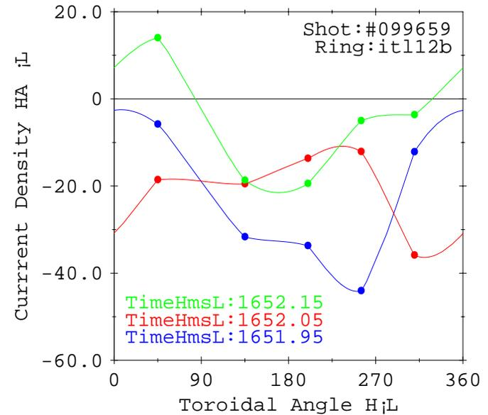
**Fig. 10** Current is strongly not axisymmetric during an ELM event, contrary to a conventional assumption. It is sometimes (as is here) ‘bi-polar,’ and flows in opposite directions from one toroidal location to another.
