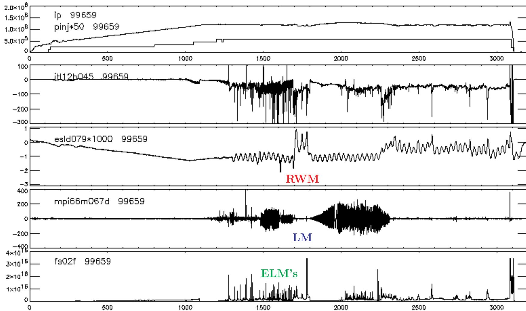
**Fig. 4** A typical discharge with many types of interesting magnetic activity: (from top)  $I_p$  and  $P_{inj}$ , Tile Current, Saddle Loop (with driven oscillations), Mirnov, and  $D_\alpha$  signals.
