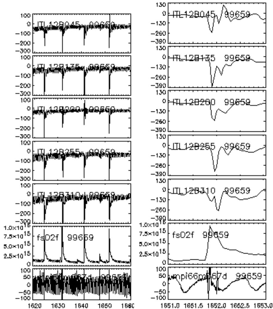
**Fig. 9** Current is small and largely axisymmetric between spikes (left), but can rise up to -400 A per tile at spikes (right).
