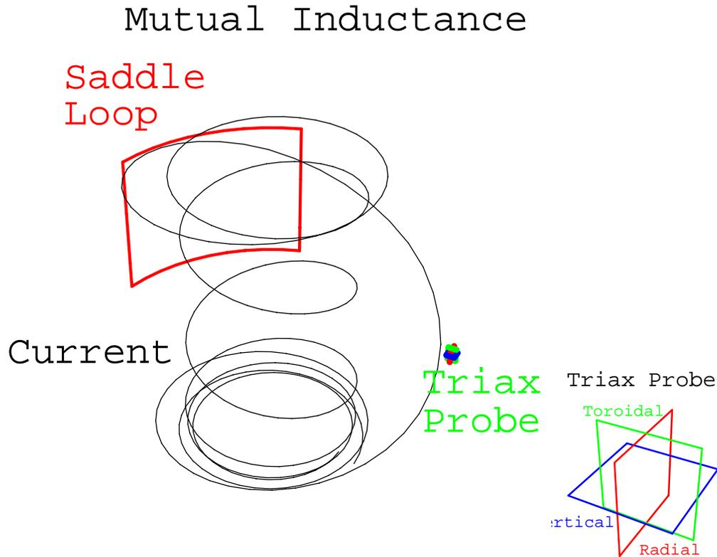
**Fig. 15** Field is determined from calculations of mutual inductance between current following a helical field line obtained from an equilibrium and magnetic sensors (actual or fictitious).
