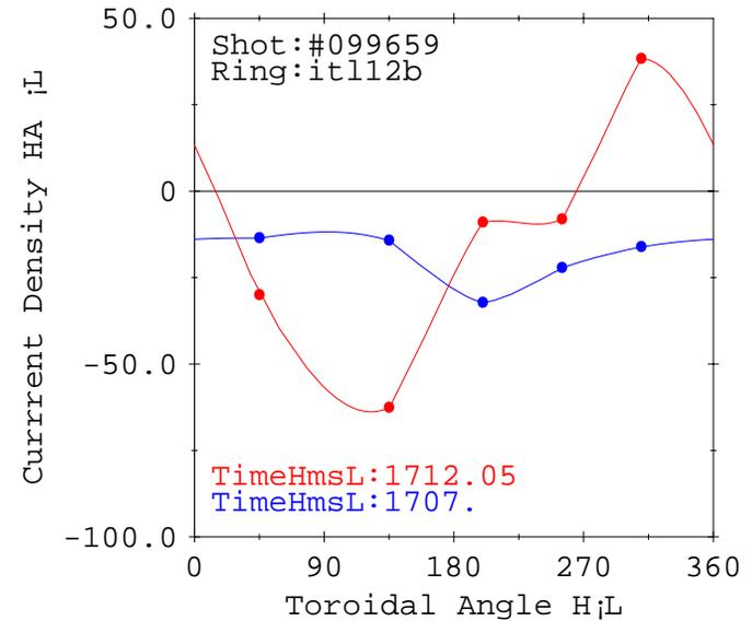
**Fig. 8** Current is ‘uni-polar’ with an axisymmetric base of around 15 A/deg and not axisymmetric toroidal variation of 15-20 A/deg. A much stronger variation up to 65 A/deg appears at spikes, where current is sometimes (as is here) ‘bi-polar,’ and flows in opposite directions from one toroidal location to another.
