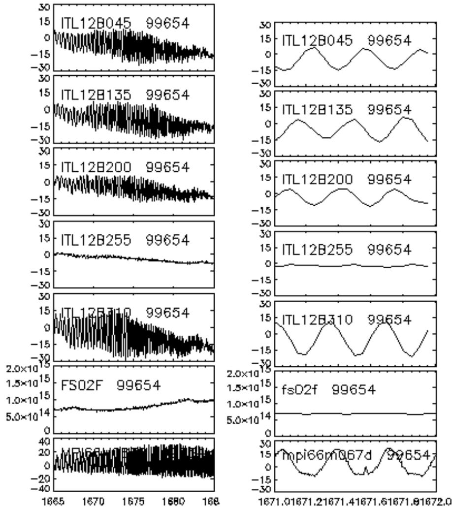
**Fig. 13** Current oscillates at the same frequency (about 3 kHz) as MHD mode, but oscillations are clearly bi-polar.
