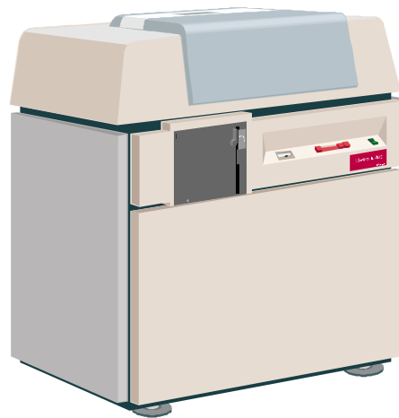
HP Magneto-optical 600fx 620 GB from 238 platters 2.3 GB/platter, 6 drives
