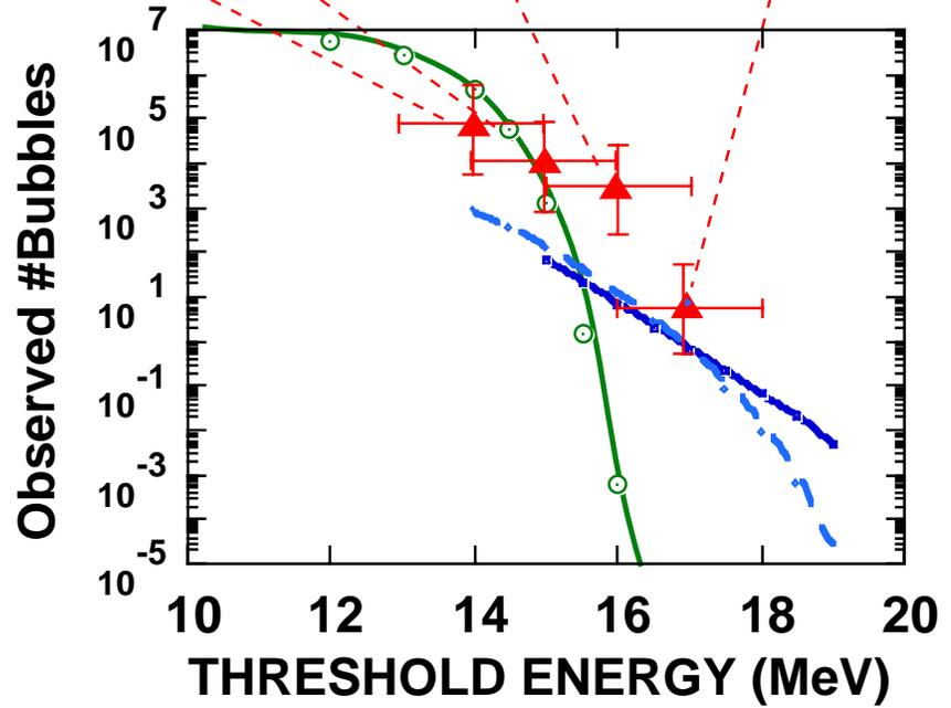
**Measured BD signals above 16 MeV are much larger than beam-beam, beam-target or thermonuclear reactions**
