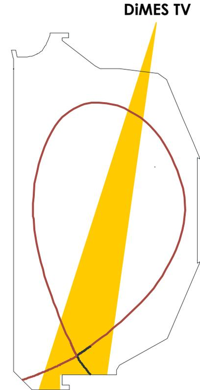
DIMITS TV, looking down in lower divertor, Mol filter 390 nm, frame rate 5 Hz, integration time 50 ms
