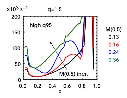
ExB flow shear at high q95 is is ~2x value at low q95.
