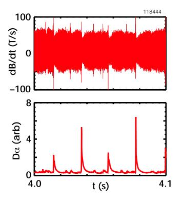
This modulation can lead to a poloidal magnetic flux pumping effect (similar to the process whereby sawteeth maintain q0 ~ 1).  Averaging over many ELMs, analysis of MSE data shows that, at an ELM, q increases inside the q=3/2 surface.
