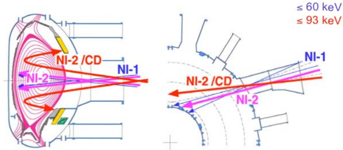
Re-direction of neutral beam injection system
