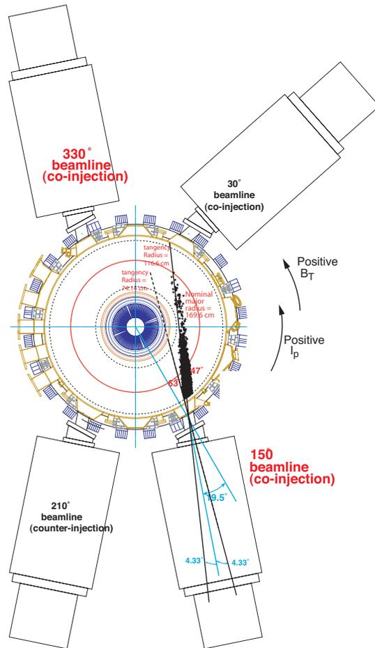
Poloidal projection of fast ion birth points on a single toroidal plane
