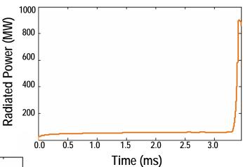
Unlike pure helium, stochastization of flux surfaces occurs sooner, produces very large radiated power spike
