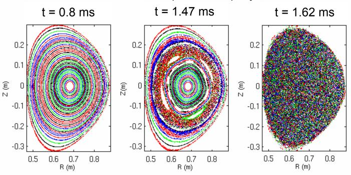
Flux surfaces are completely destroyed in this case; other simulations have shown good flux surfaces remaining inside q=1
