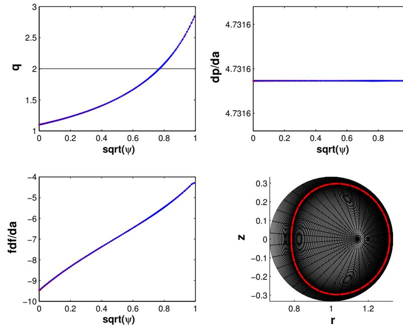
Figure 9: Toroidal equilibrium with profiles (original and fitted by TWIST-R)
