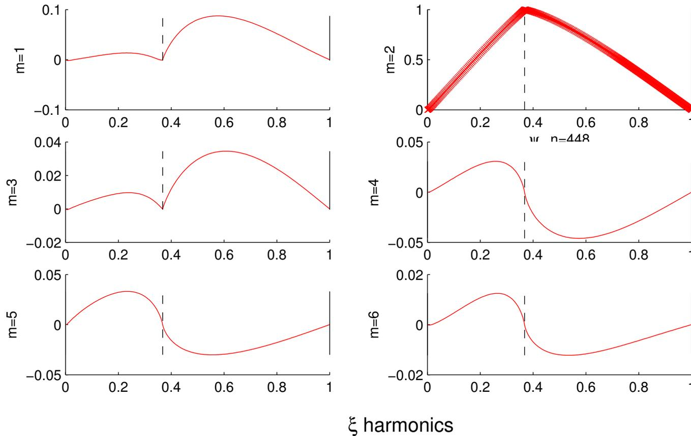
Figure 3: Poloidal harmonics for the radial component of the total displacement  $\tilde{\xi}$  with  $\mu = 1.39$
