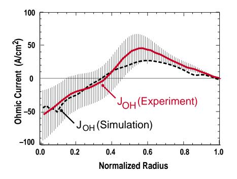
• Experimental  $J_{OH}$  from the loop voltage analysis:  $- E_{\parallel} = \frac{d\Psi_{pol}}{dt} \Rightarrow J_{OH} = \sigma_{neo} \cdot E_{\parallel}$
