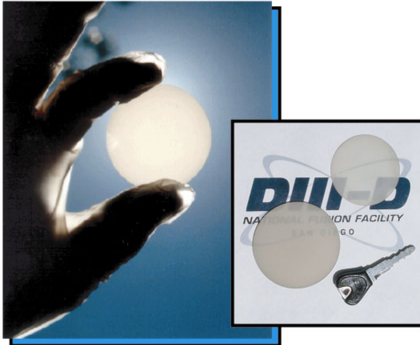
Chemical Vapor Deposition diamond disks for high power gyrotron output windows
