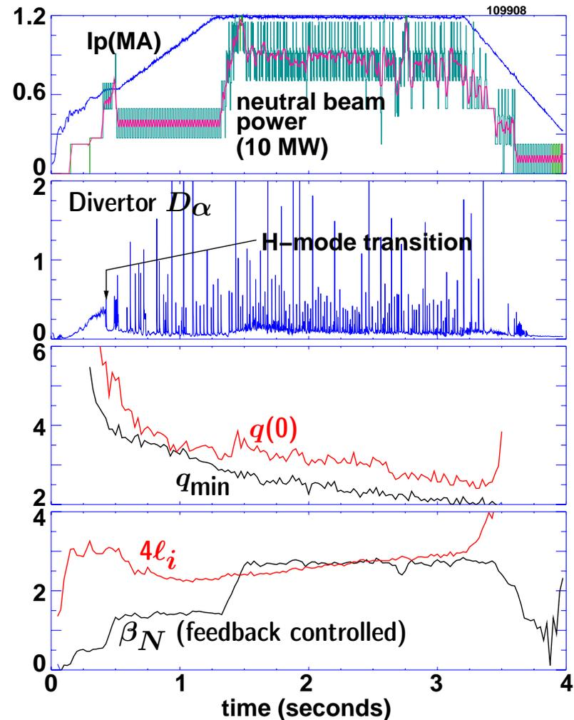
The experimental measurement of the no-wall  $\beta_N$  limit is made by observing the effect on toroidal rotation and stability as the correcting current for nonaxisymmetric error fields is removed
