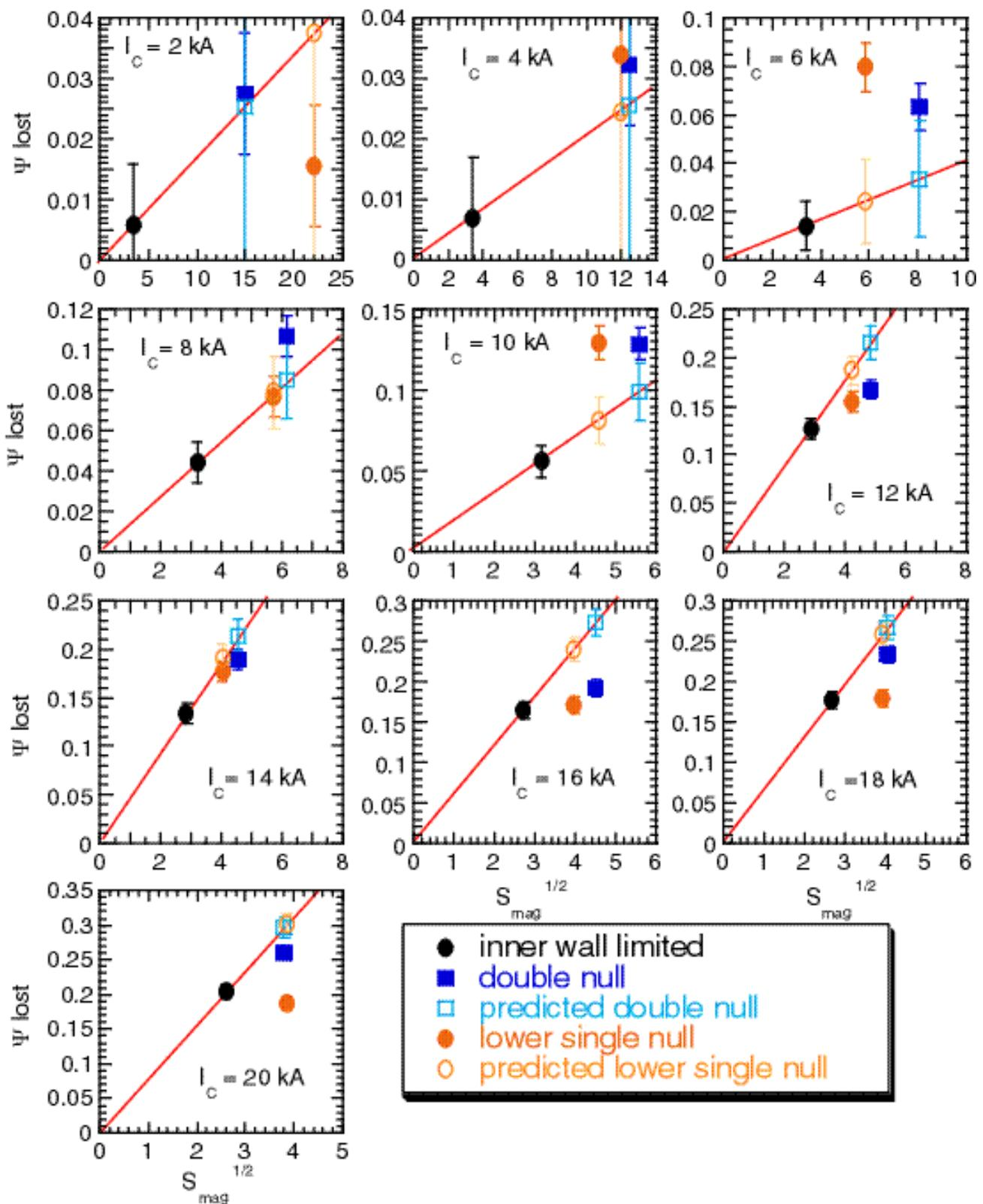
The DN shape generally fits an  $s^{1/2}$  scaling while the LSN shape deviates from the  $s^{1/2}$  scaling at high  $I_c$
