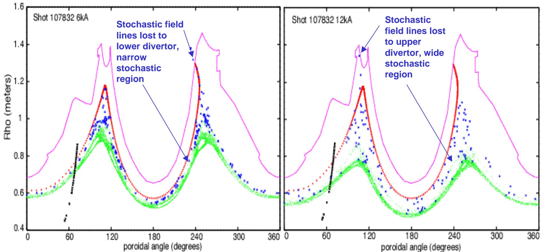
The edge magnetic flux loss is a complex function of the C-coil current, mode spectrum and plasma shape
