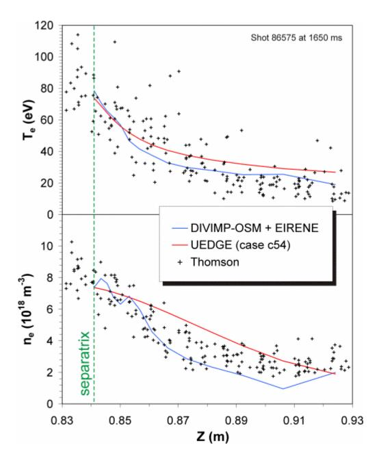
The Z coordinate is measured vertically, along the line of the Thomson laser
