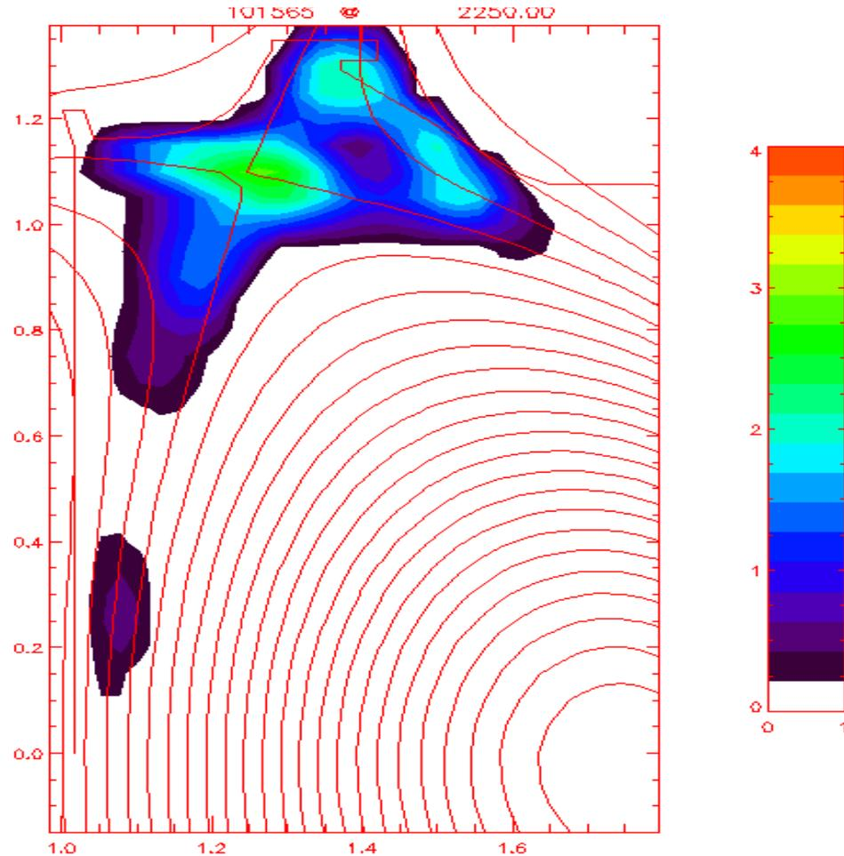
Detached closed divertor: Carbon profile localized at X-point; D<sub>g</sub> emission in far SOL and extends up divertor legs.
