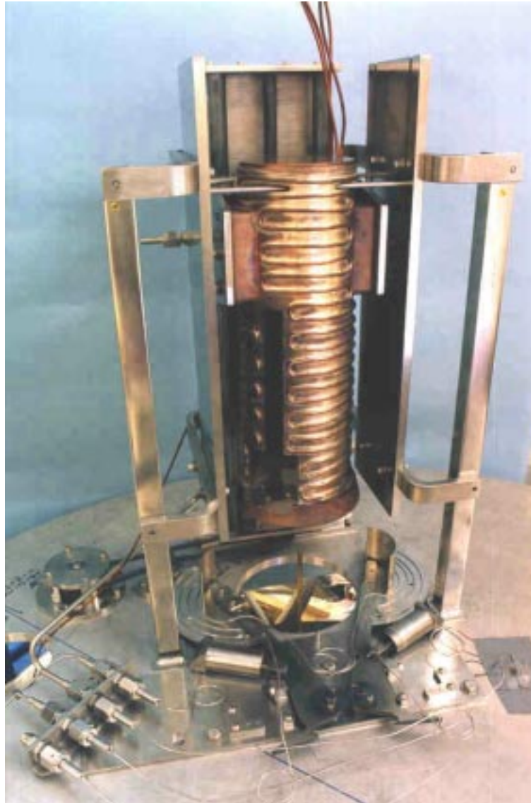
Fig. 8. Shroud cooler with lifting mechanism.
