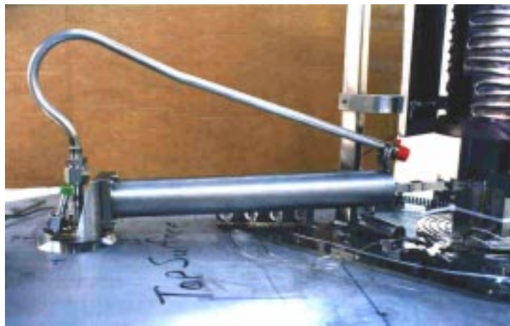
Fig. 5. Target manipulator arm with gripper and fiberscope.
