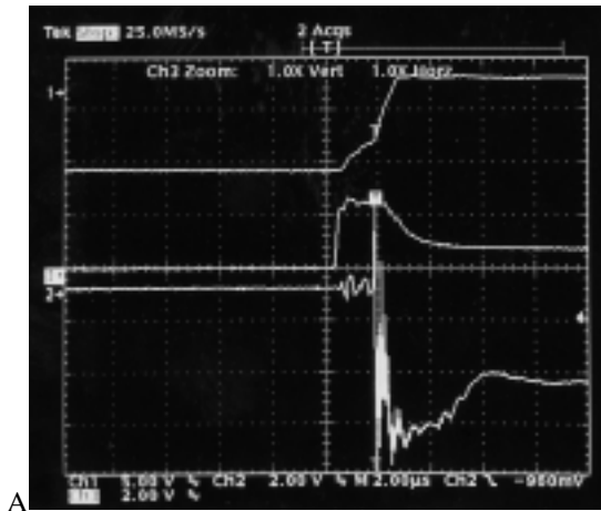
Fig. 4. Results of the crowbar wire test in which a 36 gauge wire survived repeated trials. The middle trace is the wire current (400 A/div), the bottom trace is the crowbar current (400 A/div), and the top trace is the M/R output voltage (50 kV/div).
