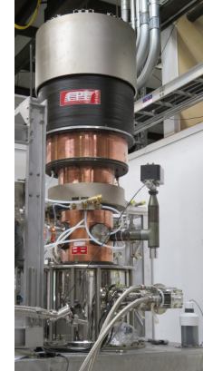
New Generation 1.5 MW Depressed Collector Gyrotron 'Vader'
