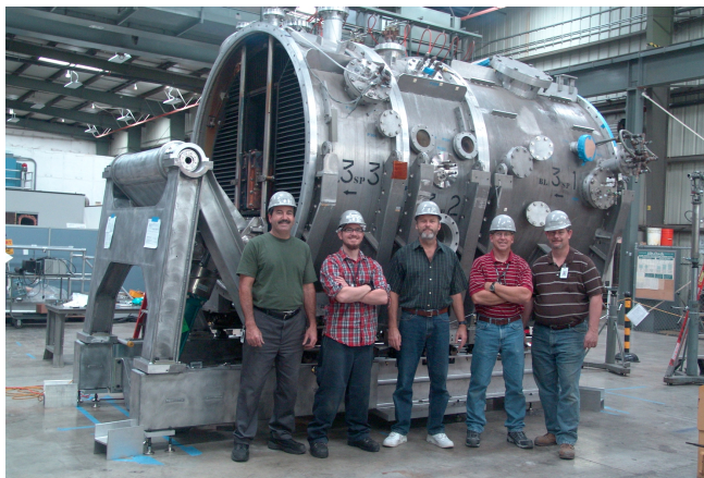
Members of the DIII-D Neutral Beam Group stand in front of a beam housing. This section neutralizes ions that then pass onward to the tokamak, while also capturing the ions that fail to neutralize.
