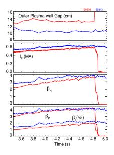
Figure 1: Comparison of two discharges with only input difference in the programmed waveform for the plasma-wall outer gap. Discharge with larger gap (red) suffers a beta collapse and disruption at  $\beta_N \sim 3.6$ . Discharge with reduced gap (blue) exceeds this  $\beta_N$  value, and sustains higher  $\beta_N$  and  $\beta_T$  values until the high heating power phase ends.
