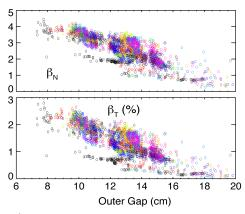
Figure 2: Database plots show plasma performance strongly improving with smaller outer gap.
