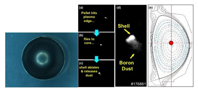
Left: X-ray image of 3.6mm-diameter,  $40\mu$ m-thick, 30mg B-filled diamond shell. Right: Visible imaging of (a) shell pellet hitting low-field-side boundary of plasma, (b) continuing through plasma toward core, (c) ablating and releasing boron dust in core. (d) Expanded view of (c), highlighting shell and dust. (e) Plasma cross-section with red dot indicating pellet location at time of dust release in (c). Injection velocity  $\approx$  230 m/s. *Image courtesy of ...*
