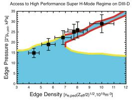
Safe passage of the DIII-D experiment (black symbols) to high edge pressure (red-bounded Super-H Mode region) requires precise navigation through operating conditions. [Courtesy of General Atomics]
