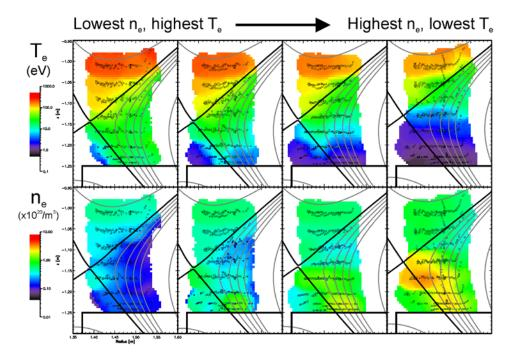
Figure 1: 2-D electron temperature (top row), and density (bottom row) for each of four plasma boundary densities increasing from left to right as measured by divertor Thomson scattering in DIII-D. Small squares indicate measurement locations mapped to the displayed magnetic equilibrium.
