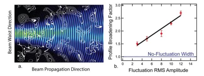
Fig: a.) Simulations find microwave beam propagation through turbulent structures of a similar scale (shown in white) leads to broadening of the RF beam. b.) A collection of different regimes on the DIII-D tokamak finds a linear relation between the edge fluctuation level and the degree of beam broadening as compared with fluctuation-free ray tracing.
