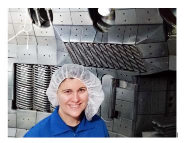
Like books leaning on each other on a partially filled shelf, the distinctively tilted 12 modules of the combline traveling wave antenna are mounted on the plasma-facing surface of the DIII-D vacuum vessel, surrounded by a picture frame of protective graphite tiles. The larger modules partly obscured by the researcher's head are another kind of wavelaunching antenna.
