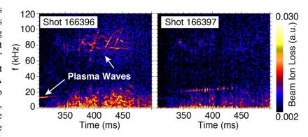
TURNING OFF TROUBLESOME WAVES: Spectrograms of measured beam ion loss. Both plasma shots feature the same total beam power, but the shot shown on the right utilizes a beam voltage program that greatly reduces the amplitude of coherent plasma waves. Adapted from D.C. Pace, et al., Nucl. Fusion 57, 014001 (2017).
