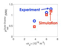
The high radiation levels found in experiment are also found in simulations (Image by ORNL)
