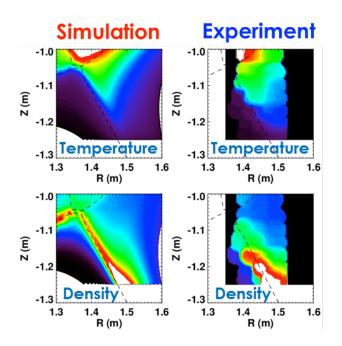
**NEW MODELING SOLUTIONS**: Simulations reproduce the plasma temperature (top) and density (bottom) in the divertor region. (Images by ORNL)
