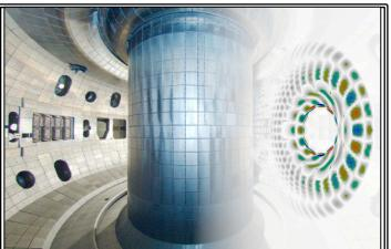
**New route to fusion energy**: Cutaway view with simulated AE structures in DIII-D tokamak at GA. AE instabilities cause fast-ions to move away from plasma core; controlling them could increase fusion performance in future reactors.
