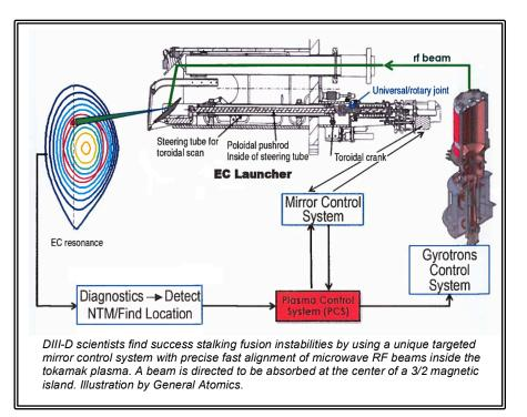
The enemies being stalked by these scientists at DIII-D are tearing modes that produce undesirable magnetic islands in otherwise toroidally symmetric tokamaks, which are complex steel-coated magnetic containers capable of containing plasma hotter than the Sun.
