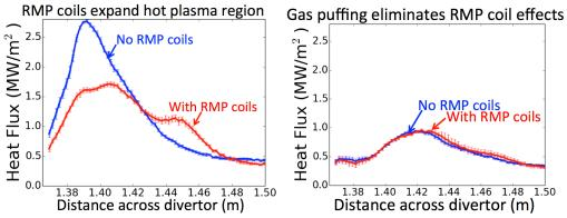
Figure 1. A slice of the heat deposited by the plasma onto the armored divertor tiles is shown for base cases in blue where no RMP coils are used and for cases with RMP coils in red (a) where little gas puffing is used and (b) where a large amount of gas puffing is seen to reduce the heat in both cases, making them nearly identical.
