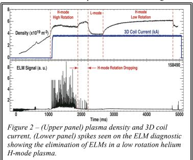
recovered and the ELMs are completely eliminated. Based on these experiments a new approach has been developed to control the power radiated by the plasma that avoids these L-mode transitions which can be applied in ITER.
