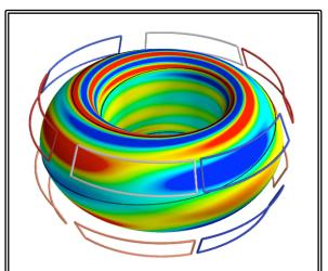
Figure 1 – Keeping energy-producing plasma in control: Simulated plasma response to 3-D perturbation coils on DIII-D produced using IPEC. Courtesy of Nikolas Logan/Princeton Plasma Physics Lab
