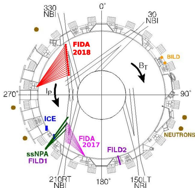
Figure 1. Topview of DIII-D fast ion diagnostics. “FIDA 2017” is obsolete. Both INPA1 and INPA2 view the 330 beamlines.
