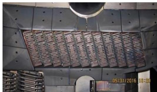
Fig. 2-59. The low-power prototype comb-line traveling wave antenna as installed in DIII-D during the 2016 campaign.
