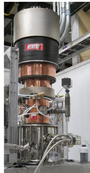
*Fig. 5-5. The first 1.5 MW gyrotron was delivered and installed in its socket in mid FY17.*
