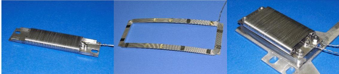
*Fig. 6-3. a) Poloidal magnetic probe. b) Radial field saddle loop c) Compact combined poloidal and radial magnetic probes.*
