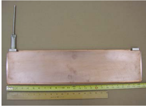
Fig. 5-7. Prototype micro-channel cooling module utilizes parallel water flow through multiple molybdenum flow channels to provide active cooling of the pole shield.
