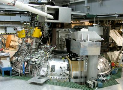
R<sub>0</sub> = 1.5 m, a = 0.51 m, I<sub>p</sub> < 600 kA B<sub>T</sub> ~ 3-4 kG, n<sub>e</sub> ~ 10<sup>19</sup> m<sup>-3,</sup> T<sub>e0</sub> < 1.3 keV  $\tau_E$  ~ 10 ms, β =/B<sup>2</sup>(a)=15%
