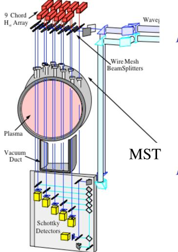
$Interferometer \longrightarrow \tilde{n}$   $\phi \sim \int n dl + \int \tilde{n} dl$   $Differential Interferometer \longrightarrow \nabla \tilde{n}$  $\frac{\Delta \tilde{\phi}}{\Delta x} \quad \Delta x \sim 1 mm$
