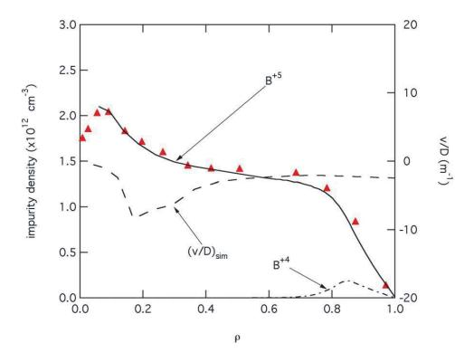
Here is shown a simulation of B<sup>+5</sup> density (solid line) and B<sup>+4</sup> density (dash-dot line) compared with the measured B<sup>+5</sup> density (▲). v/D (dashed line) required in the simulation is plotted on the right axis.
