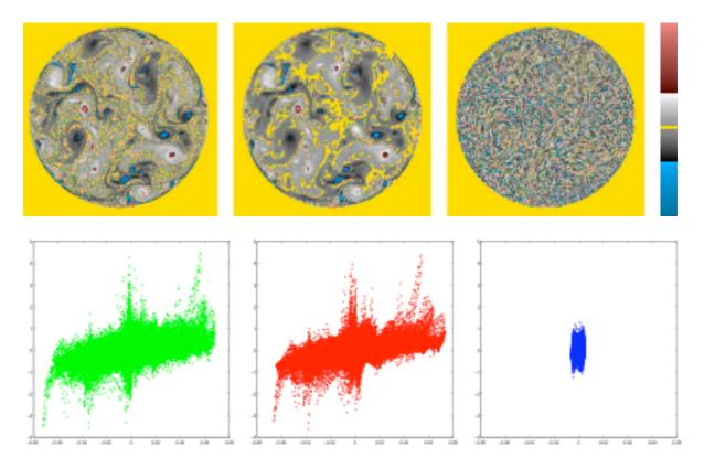
**Top :** total (left), coherent (center) and incoherent (right) vorticity fluctuations of a twodimensional fully-developed turbulent flow of zero mean, which has been computed by direct numerical simulation of the two-dimensional Navier-Stokes equations. **Bottom :** scatter-plot between vorticity and stream function which characterizes the presence of coherent structures in the total and coherent, but not in the incoherent fluctuations.
