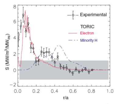
Mode converted electron heating profile from ICRF in C-Mod
