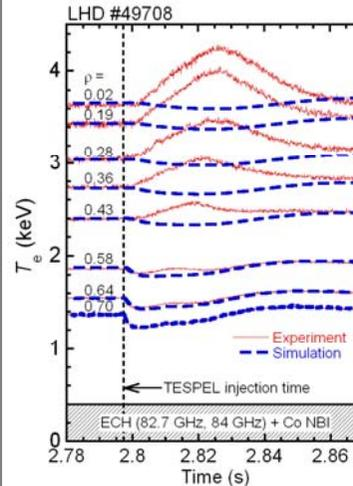
✓ Edge cooling experiment of LHD shows a significant rise of core  $T_e$
