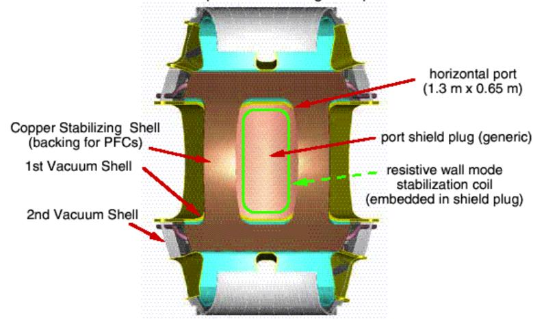
Wall stabilization required to attain full Advanced Tokamak potential.
