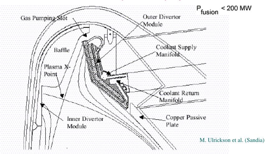
Reference plan is semi-detached operation with <15 MW/m<sup>2</sup>
