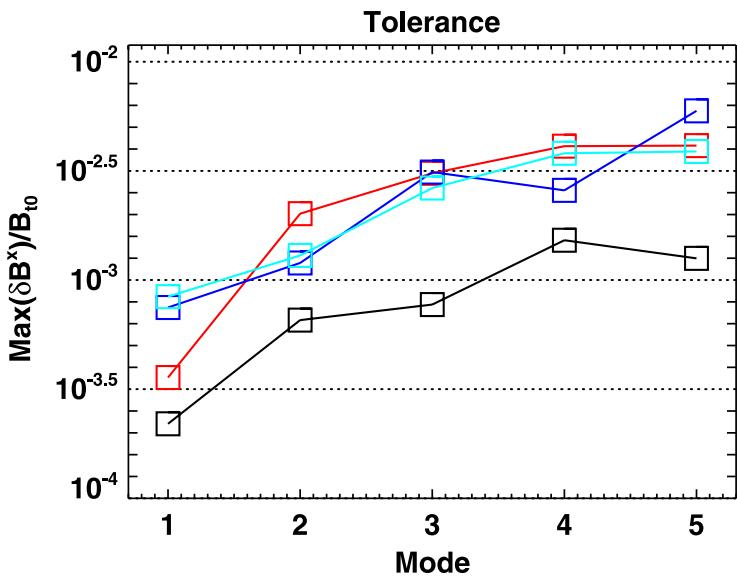
Island drive in ITER,  $\propto 1/\sigma_i$ , for  $n = 1$  (black),  $n = 2$  (red),  $n = 3$  (blue) and  $n = 4$  (light blue). For all rational surfaces  $q=m/n$  and for three ITER equilibria (*inductive, hybrid, advanced*).
