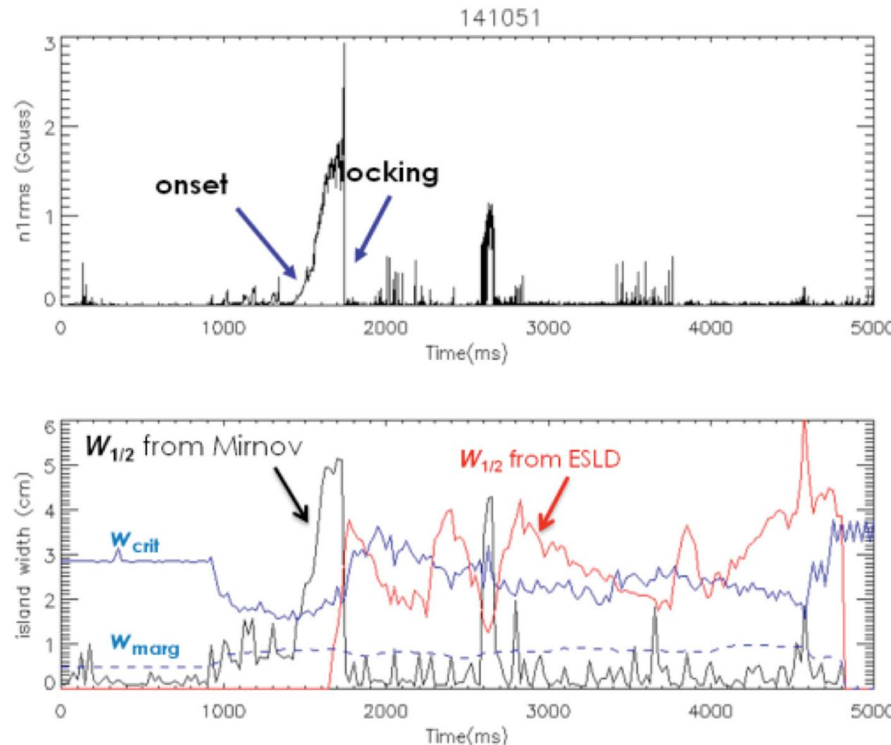
And should unlock when width below critical, but changes of NBI torque need to be included in the analysis
