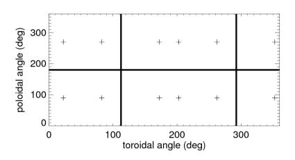
As a result, the radial magnetic field as a dominant m=1, n=-7 harmonic, plus m=0,1,2, n=-7 harmonics to represent the radial field perturbation localized at the toroidal gap
