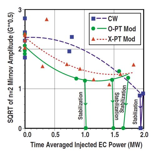
Modulated ECCD more stabilizing than CW
