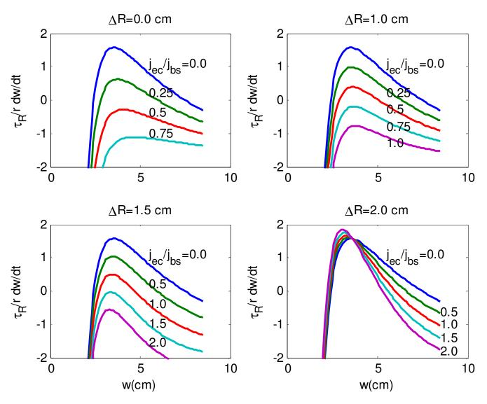
Normalized island growth rate for parameters typical of DIII-D discharges associated with the m/n = 3/2 NTM and unmodulated current drive.
