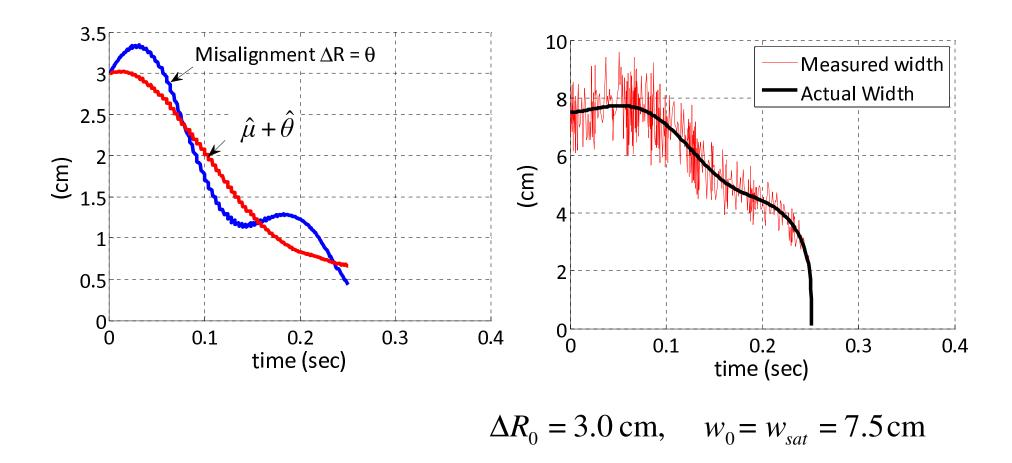
If the initial step direction is unknown the average suppression time is m = 0.25s with standard deviation  $\sigma < 0.01s$  for continuous current drive.
