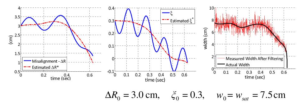
Standard Extremum Seeking algorithm with two parameter optimization  $(\Delta R, \xi)$ : The average suppression time is m = 0.62s with standard deviation  $\sigma = 0.10s$ .
