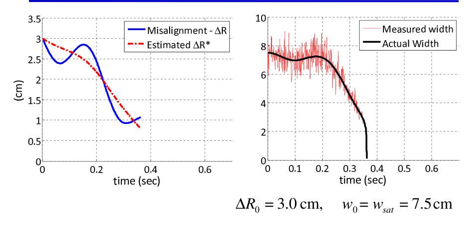
Modified Algorithm: Use gain scheduling to modify the gain  $\gamma$  as a function of the island width. For continuous current drive the average suppression time is m=0.40s with standard deviation  $\sigma=0.07s$  and m=0.41s,  $\sigma=0.13s$  for 50/50 duty-cycle current drive centered at the O-point.
