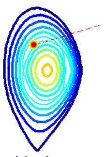
The plasma rotates around the torus. As a result the island structure rotates in a fixed cross-section. Current driven in the center of the island around the O-point has the highest stabilizing effect. Current driven outside of the island or around the X-point has a destabilizing effect. Thus it is beneficial to modulate the beam in sync with island rotation to deliver current around the O-point.
