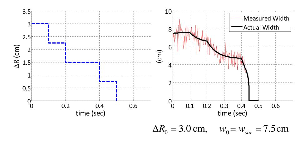
If the initial step direction is unknown the average suppression time is m = 0.62s with standard deviation  $\sigma = 0.14s$  for continuous current drive and m = 0.50s,  $\sigma = 0.18s$  for 50/50 duty-cycle modulated current drive centered at the O-point.
