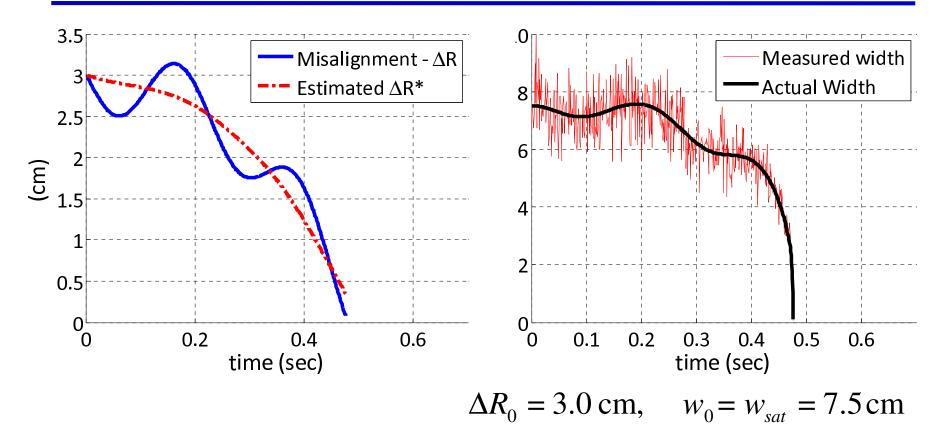
For continuous current drive the average suppression time is m = 0.54s with standard deviation  $\sigma = 0.06s$  and m = 0.44s,  $\sigma = 0.10s$  for 50/50 duty-cycle current drive centered at the O-point. There is a notable improvement in average suppression time as well as consistency over the search and suppress algorithm.
